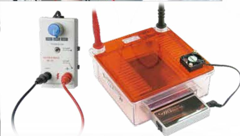
Specifically designed for DNA and RNA electrophoresis.
