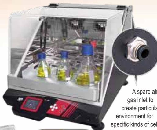
A spare air/gas inlet to create particular environment for specific kinds of cell/microbial
