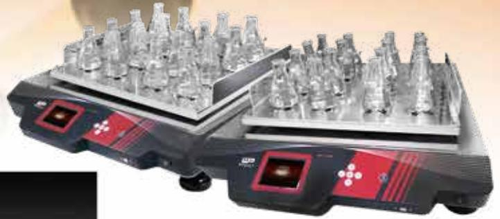
The WS-200 shaker is developed to offer an integrated solution for every mixing requirement. With a large 18.1"X18.1" platform and a wide selection of labware holders, this versatile machine can accommodate five 2L flasks or any combination of labwares up to 30kg. This powerful machine is equipped with a maintenance-free brushless DC motor that permits the device to operate noiselessly even at 500rpm under programmable mode of operation or continuous mode up to 999hr.
